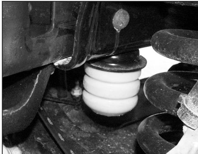
21. Position the cup on the provided bump stop extension. (01001) The alignment tab on the bump stop cup will fit in the second hole in the extension
