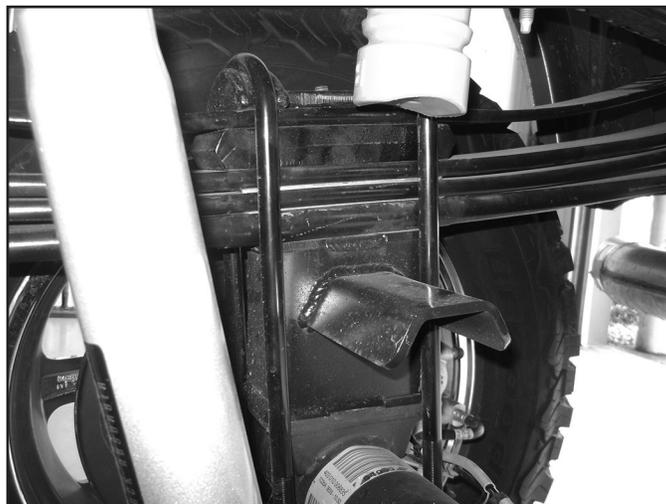
82. Raise the axle to engage the block spring alignment pins. Fasten the entire assembly with the provided u-bolts, washers, and nuts. Snug but do not torque the u-bolts at this time. (Fig 2)
