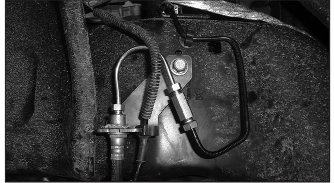
63. **6" Kit Only:** Attach the ABS wire to the new brake line bracket. The rubber grommet may need to be slid up the ABS line, use silicone spray to help aid in moving the rubber grommet. (Fig. 25)
