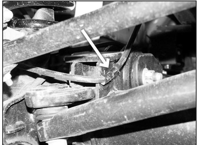
9. Disconnect the upper sway bar end links from the sway bar. Push the sway bar up out of the way. Retain hardware.
