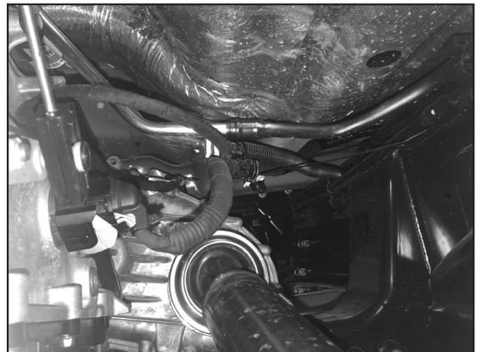
28. The OE radius arm bracket will need to be trimmed for upper arm clearance. Use the forward hole as a reference and draw a horizontal and vertical line. Cut along the marked lines to remove the forward section of the OE radius arm mount. Perform this same cut on the inside surface of the radius arm mount as well. (Fig 11)
