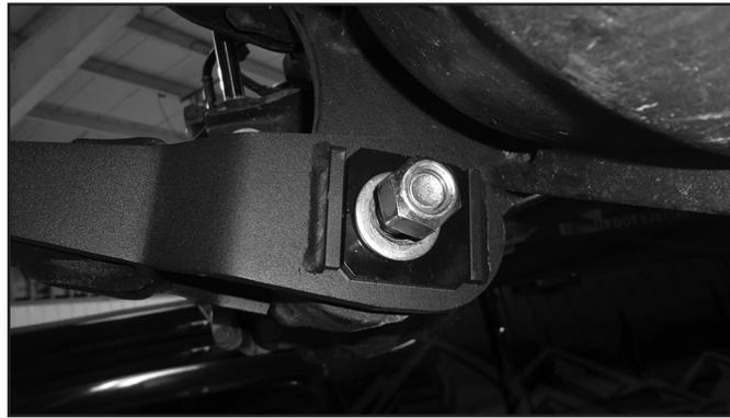
41. Use the provided 1/4" bolt, 1/4" SAE washers, and 1/4" nut with wire clamp from Bolt Pack BP1071 to attach the hub actuator hose to the upper control arm in order to keep it away from the bump pad on the axle. Torque this hardware to 76 in-lbs.
