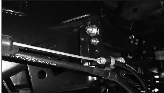
102. Install the passenger side E-brake cable into the bracket, make sure the tabs on the cable lock the cable into place. (Fig. 7)
