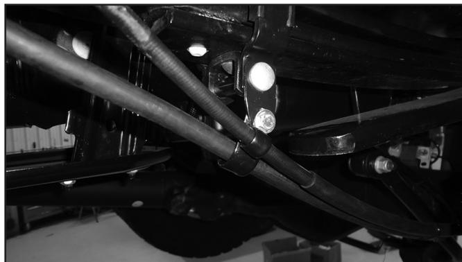
104. Use the two provided wire clips from bolt pack 989 to secure both E-brake cables to the E-brake clamp bracket with the provided 5/16" hardware from bolt pack 989.
