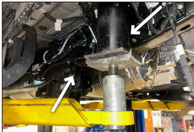
36. Insert a carriage bolt plate onto the fish wire and then thread a 1/2" carriage bolt onto the fish wire. Feed the carriage bolt plate into the frame and pull the fish wire with carriage bolt through until the threads are exposed. Unthread the fish wire from the carriage bolt. Lightly install a 1/2" SAE Washer and 1/2" prevailing torque nut onto the threads being careful not to push the bolt into the vehicle's frame rail. (Fig.. 18A, 18B)
