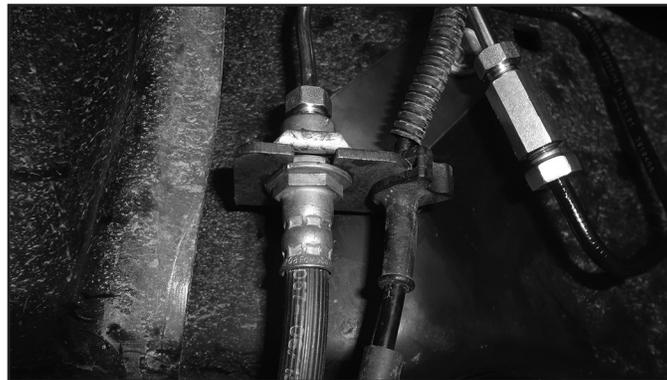
64. **4" Kit Only:** Install the new brake line brackets, the brackets are side specific. Brake lines will need to be reformed to reach the new mounting position. It may be necessary to slightly twist the brake line fittings in relation to the hard line to get adequate clearance to the frame / wheel and tire. Attach the ABS wire to the driver's side with 1/4" hardware and cable clamp in Bolt Pack 341 (Fig 26A, 26B)
