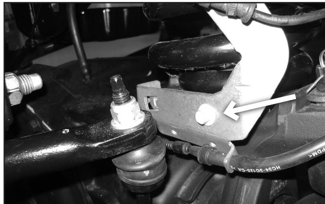
7. Remove the bolts attaching the front brake lines brackets to the frame and save the hardware (Fig. 3). Attempt to not bend the brake lines as much as possible. Remove the ABS line from the brake line bracket.
