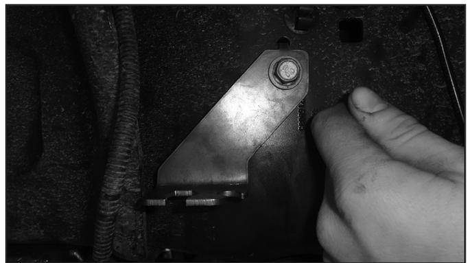
57. **6" Kit Only:** Remove the clip holding the brake line to the factory bracket. Save the clip for later installation.
