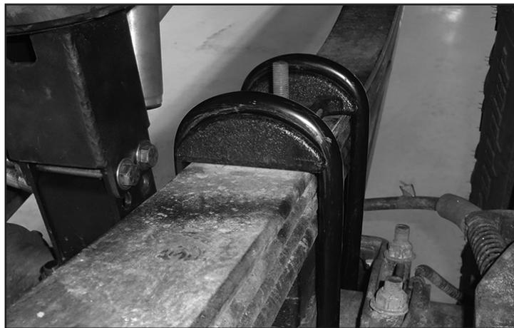
98. Install the new spring in the vehicle with the OE bolts. Use the provided 7/8" SAE Washers as spacers as needed for the front leaf spring bushing (use one on each side of the leaf spring bushing). Leave hardware loose. All of the spring pivot bolts will be torqued with the weight of the vehicle on the springs.
