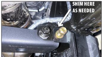
32. Drill a 9/16" hole in the frame through the hole in the side of the four link bracket. Paint the raw exposed metal. Insert the 1/2" x 1-1/4" bolt and 1/2" SAE washer from Bolt Pack BP1070 through the hole and attach using the provided 1/2" prevailing torque nut and 1/2" SAE washer. Leave hardware loose. (Fig. 15)
