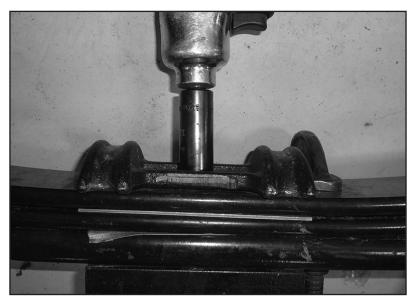
97. The OE upper U-bolt mount will be installed on the new leaf springs. Clamp the top and bottom of the new leaf springs near the center pin, but still allowing enough room to install the OE upper U-bolt mount. Remove the center pin from the new leaf springs and attach the OE upper U-bolt mount to the new leaf springs with the center pin. A pair of new center pins are provided incase the center pins in the new leaf springs strip out. (Fig. 5)
