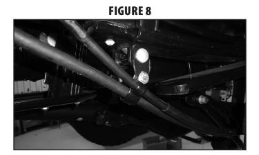
104. Use the two provided wire clips from bolt pack 989 to secure both E-brake cables to the E-brake clamp bracket with the provided 5/16" hardware from bolt pack 989.
