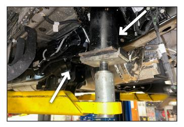
36. Insert a carraige bolt plate onto the fish wire and then thread a 1/2" carriage bolt onto the fish wire. Feed the carraige bolt plate into the frame and pull the fish wire with carriage bolt through until the threads are exposed. Unthread the fish wire from the carriage bolt. Lightly install a 1/2" SAE Washer and 1/2" previaling torque nut onto the threads being careful not to push the bolt into the vehicle's frame rail. (Fig.. 18A, 18B)
