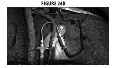
63. 6" Kit Only: Attach the ABS wire to the new brake line bracket. The rubber grommet may need to be slid up the ABS line, use silicone spray to help aid in moving the rubber grommet. (Fig. 25)
