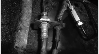
**64. 4" Kit Only:** Install the new brake line brackets, the brackets are side specific. Brake lines will need to be reformed to reach the new mounting position. It may be necessary to slightly twist the brake line fittings in relation to the hard line to get adequate clearance to the frame / wheel and tire. Attach the ABS wire to the driver's side with 1/4" hardware and cable clamp in Bolt Pack 341 (Fig 26A, 26B)
