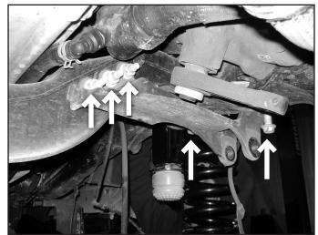
14. Disconnect the steering drag link from the pitman arm. Remove the cotter pin and castellated nut cap. Remove the nut and thread back on by hand a couple turns. Strike the end of the pitman arm near the drag link end to dislodge the taper from the pitman arm (Fig. 6). Remove the nut and the drag link from the pitman arm. Retain hardware.
