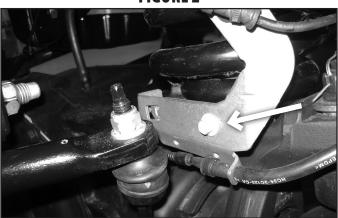
Remove the bolts attaching the front brake lines brackets to the frame and save the hardware (Fig. 3). Attempt to not bend the brake lines 7. as much as possible. Remove the ABS line from the brake line bracket.
