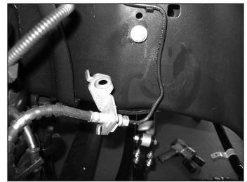
8. Free the hub vacuum lines from the axle/ radius arm to allow for adequate droop (Fig. 4A & 4B).
