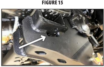
33. Mark and drill out to 9/16" the upper frame mount hole in the frame mount bracket. Paint the raw exposed metal. (Fig. 16)
